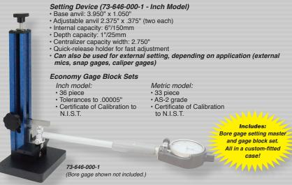
Order Number 73-646-000-1 73-646-010-0 Description Bore Gage Setting Master Kit Metric Bore Gage Setting Master Kit
