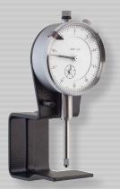
Dial Gage is designed to check wearing of disc rotors. Also used to determine deviation in thickness of rotors as well depth of disc-scoring caused by worn brakes.
