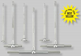
Another great tool for easy and accurate measurements. Under spring tension, the plungers of the gage expand from the center to the size of the hole being measured and are then locked in place using the knurled knob. Final hole size is obtained by measuring over the contacts with a micrometer or vernier caliper.
